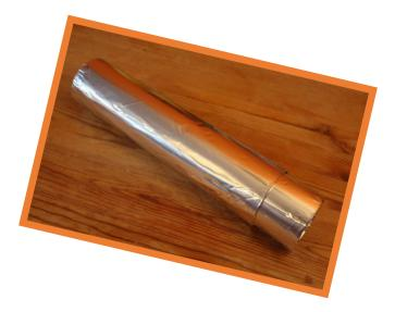
Slot the smaller tube into the larger one. You should be able to side the tubes back and forth as if you are focusing your telescope.
